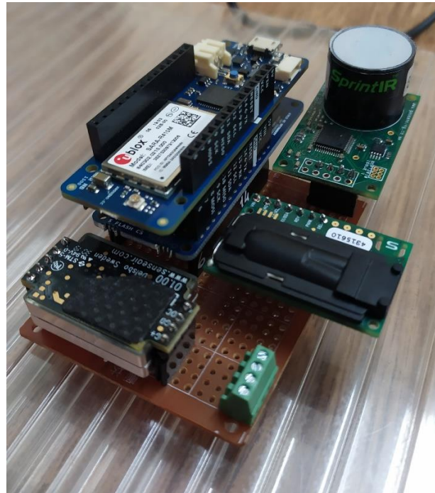
Figure 13. PCB -S8-SCD30-SprintIR-MKR1500 NB IoT microcontroller saving data on SD card
