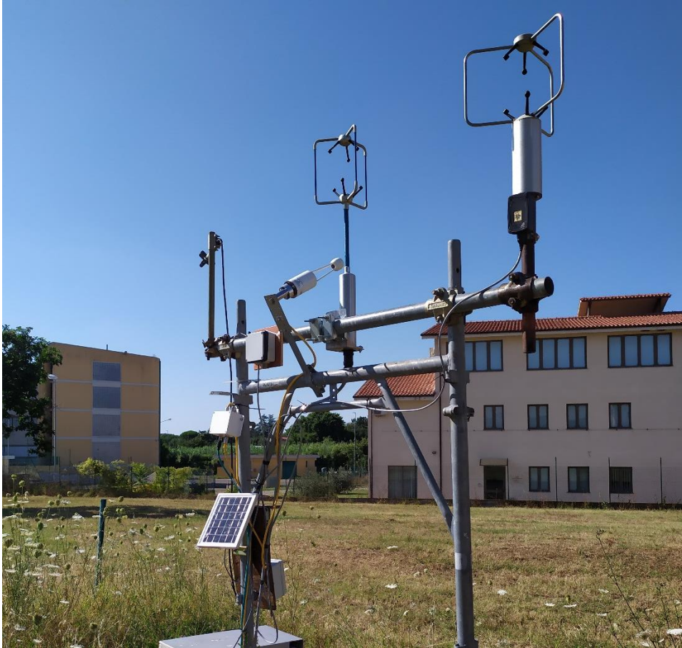
Figure 28. Installation of SprintIR and Trisonica with a standard EC system for reference
