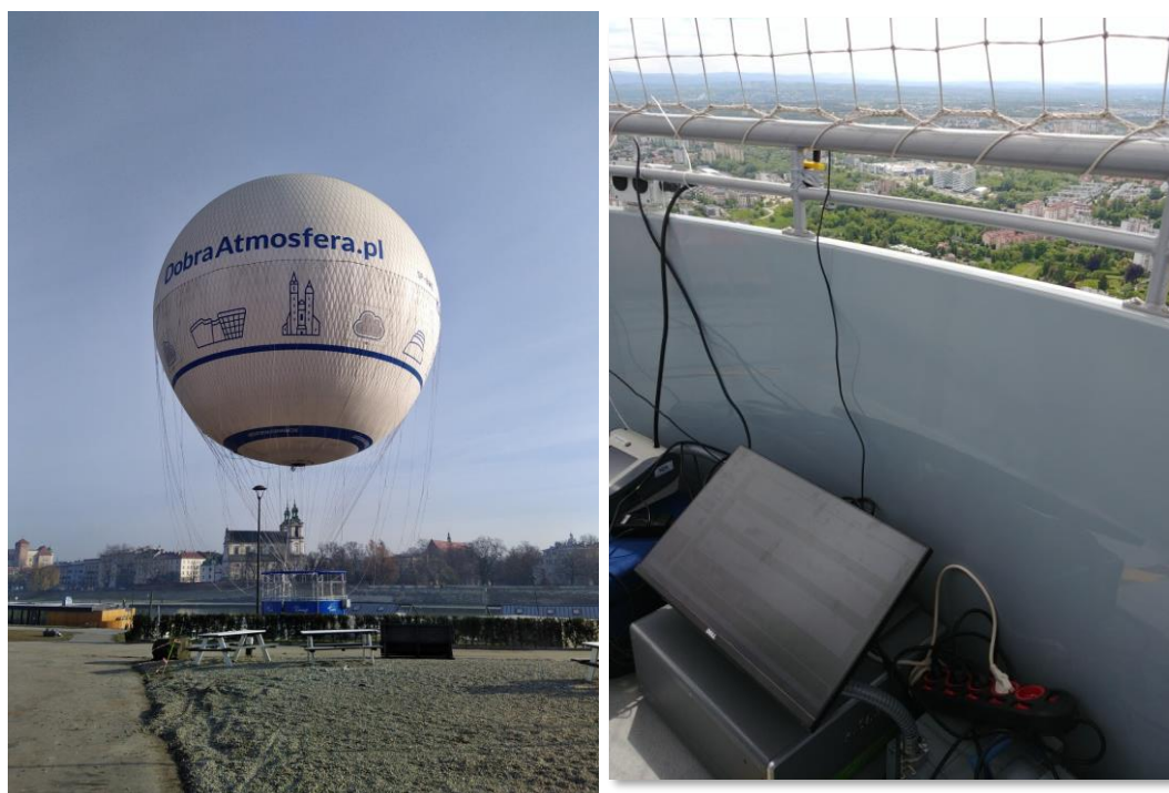
Figure 6 An overview of the tethered balloon platform (left) and the location of the measurement equipment in the balloon gondola (on the right).
